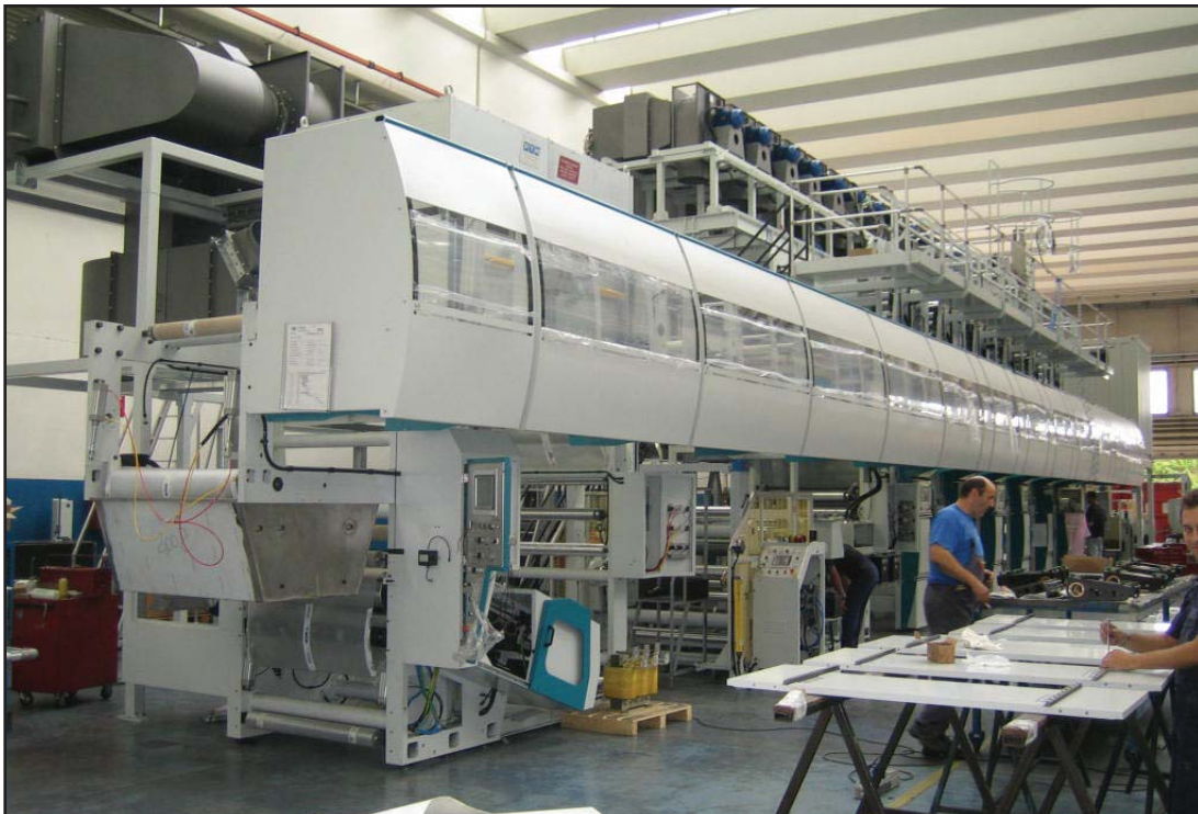
The new M-Press during production in Uteco's manufacturing facility in Verona, Italy
